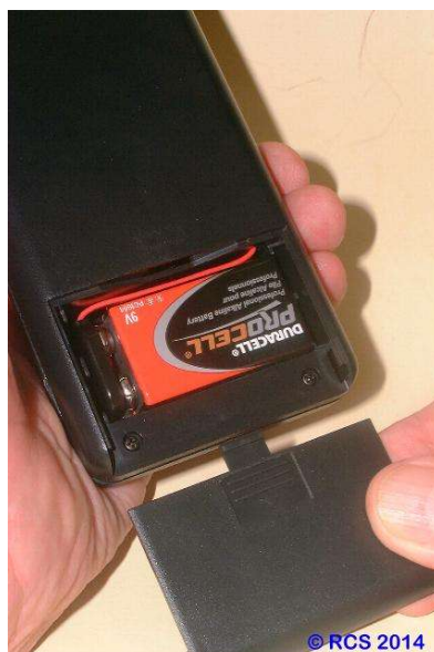
REMOVE REAR OF TX-6 TO INSERT THE 9 VOLT BATTERY. LED BLINKS WHEN BATTERY LOW. A HIGH QUALITY 9V SNAP IS USED.
