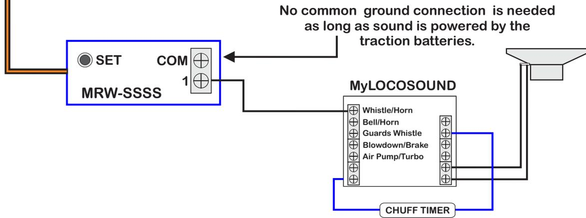
Max 2 amp load on each trigger.
