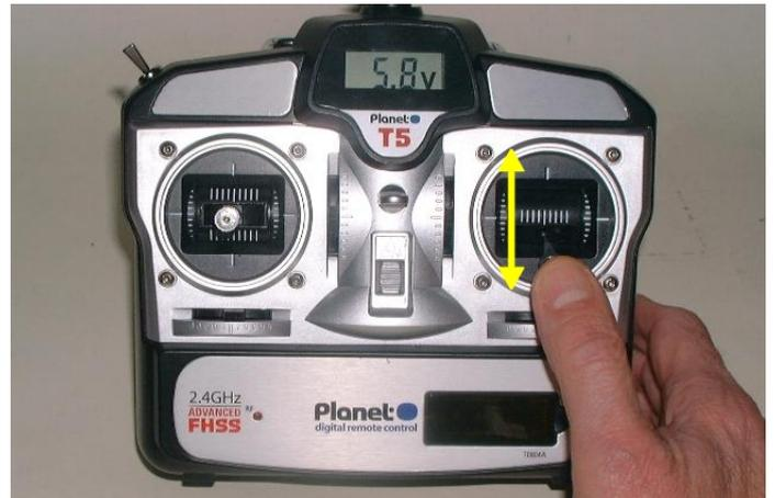
**2.4** From zero (down position), gently stroke the Throttle stick backwards & forwards full travel a couple of times. Pause briefly (less than 1 second) at end of each stroke. Then return stick to zero (down position).
