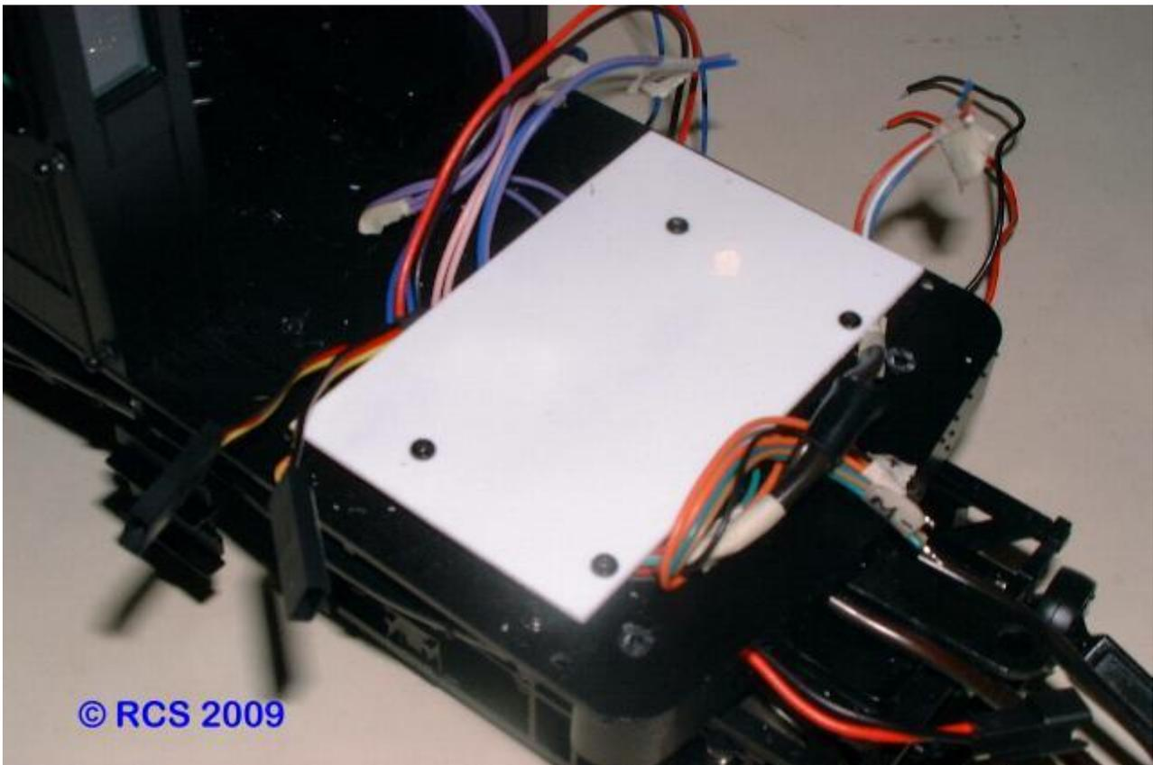
The two part RCS # PRO-6B ESC was stuck to the styrene platform with silicone adhesive. Next to these two items is the Phoenix P8 sound system. There is just enough room for all three items to fit side by side. Ensure the screw heads holding the platform don't touch the back of the ESC.
