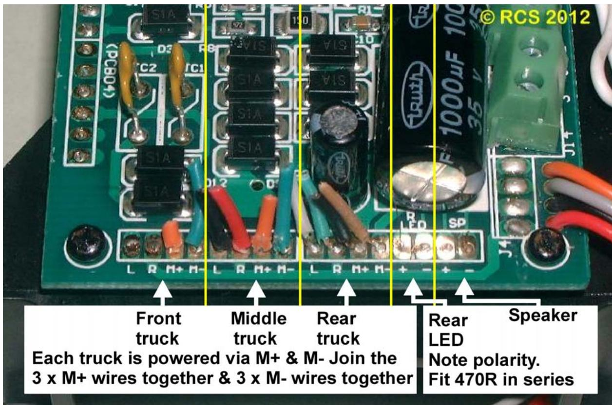
Colour wise Bachmann have correctly wired the front and rear trucks, but managed to use incorrect colours for the third truck. Be extra careful when selecting which wires to bundle. Match M + with M + only. Likewise only join M - with M - wires as indicated above.
