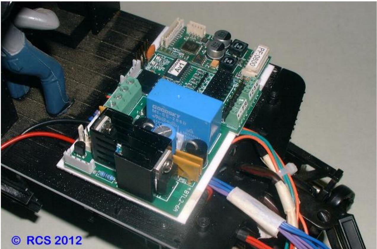
I used the slide out coal load front to mount the RCS programming pushbutton, P8 volume control & programming jack.
