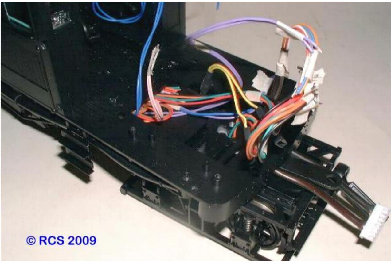
Then I made a styrene plate upon which I could mount the RCS components.
