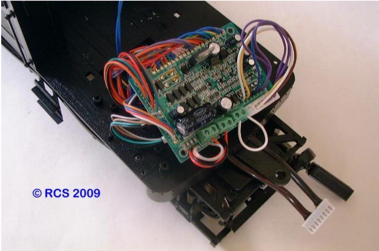
I removed all the wiring from the pcb, bundled the various common wires together and tagged them. Following are guides as to which wires are saved for later use.
