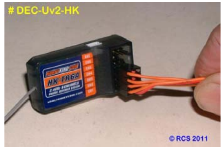
Insert the 1 x 3 way servo cable & four single wire cables into the TR6a RX. Connect as per the chart below.
