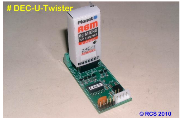
Then gently press onto socket. The fit will be tight. Do not force.
