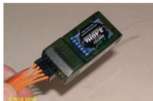
Insert the supplied servo cables into the servo sockets on the RX. 3 x wire lead to # 1.
