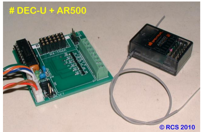
Remove the # EX-LD & binding plug before installing the RX into the # DEC-U . # DEC-U & AR-500 RX shown. The BATTERY – BIND terminals must NOT be connected.
