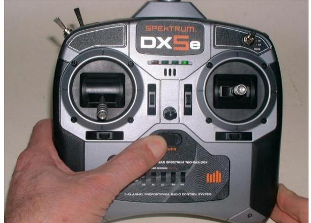
**2.2** Set the DX5e Mode # 2 channel # 5 switch on the TX to # 1 ON, i.e. pull switch towards you.
