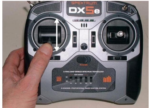
**2.4** From zero (down position), gently stroke the Throttle stick backwards & forwards full travel a couple of times. Pause briefly at end of each stroke. Then return stick to zero (down position).
