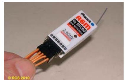
Insert the supplied servo cables into the servo sockets on the # **R6M** RX.
