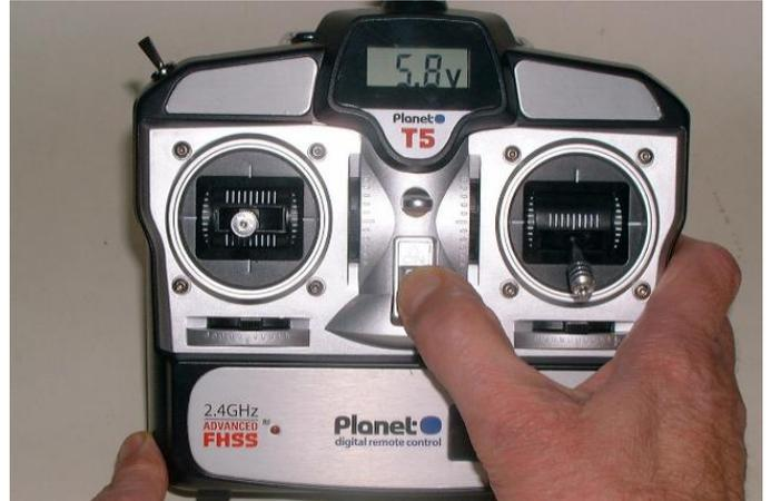
**2.2** Set the Mode # 1 T5 channel # 5 switch on the TX to "0" ON, i.e. push switch away from you.
